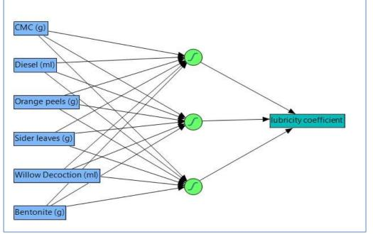
Fig. 11 Neural network analyzing the impact of the lubrication factor on drilling mud.
