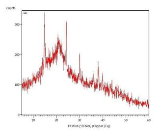
Figure 6: XRD analysis for Crushed palm leaves.
