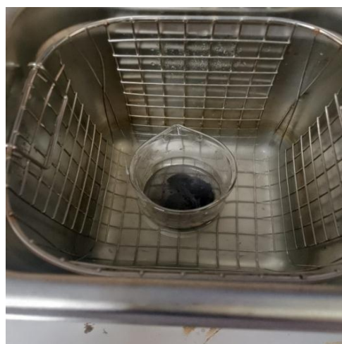
Figure 2: Sample inside ultrasonic for particle dispersion (5 min treatment, controlled temperature).
