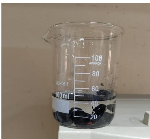
Figure 1: Initial appearance of black powder–solution mixture before ultrasonic treatment.
