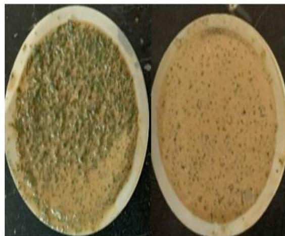
Figure 8: mud cake for Crushed palm leaves.
