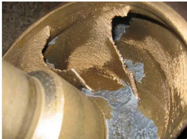
Figure 3: Worn impeller due to cavitation [6].
