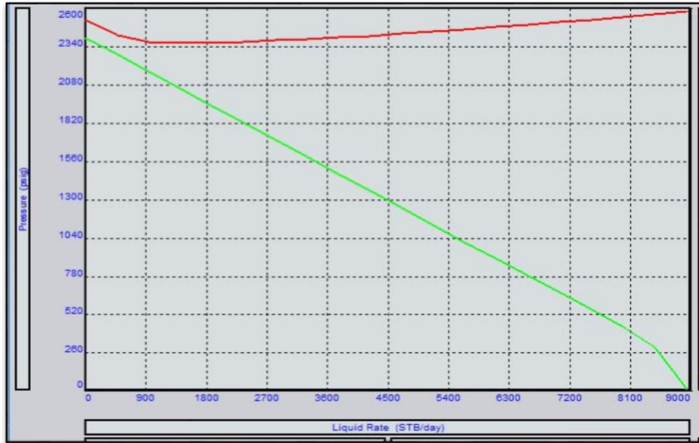
Figure 1 : Nodal analysis of well K22 from initial state
