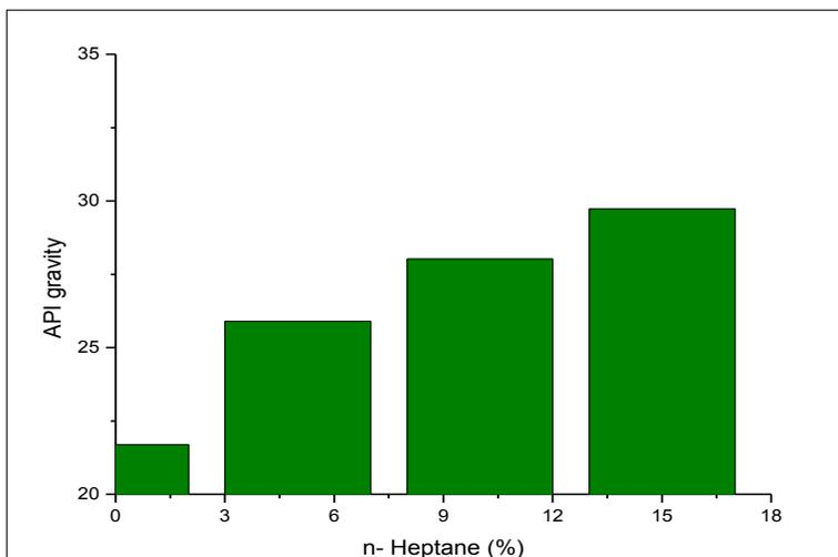
**Figure 4.** Effect of solvent concentration on API gravity.
