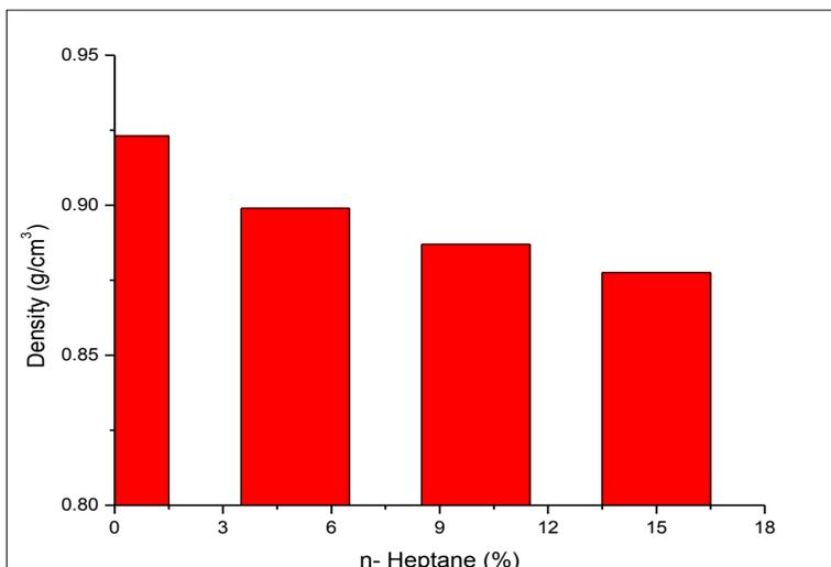
**Figure 3.** Effect of solvent concentration on density.
