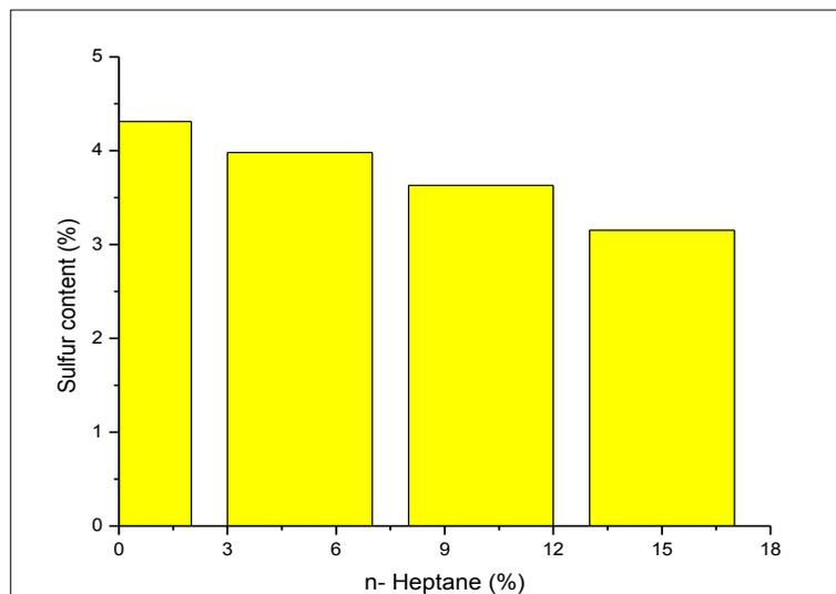
**Figure 2.** Effect of solvent concentration on sulfur content.
