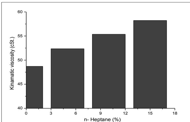
**Figure 5.** Effect of solvent concentration on kinematic viscosity.
