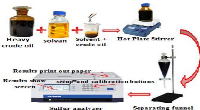
Fig. 2: Schematic Diagram of the Caustic Method's Experimental Setup
